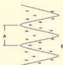
Non-radial wedge pleats have unequal air exit (D) and air entering (C) areas, which cause higher resistance and uneven usage of media.
